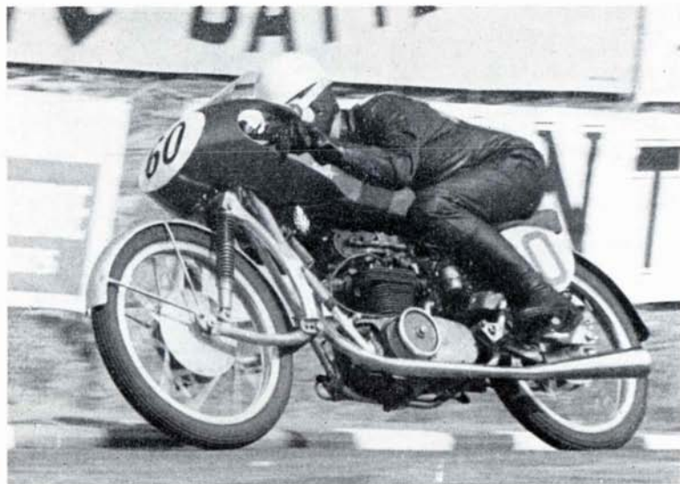
Les Graham accelerating out of Governor's Bridge dip on his 125 c.c. M.V. Note how the cowling blends with the rider's body. (Photo: Salmond)
