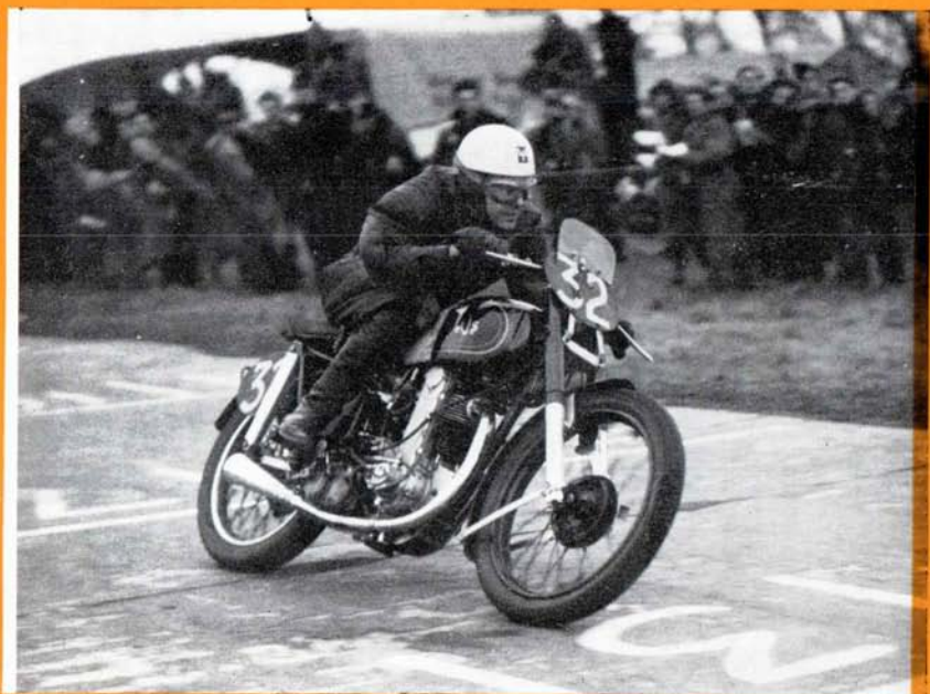
E. N. IFFLAND winning the A.J.S. Race at Haddenham, June 4th, 1949. His 346 c.c. machine is a pre-war model, owner tuned and fitted with Telescopic Forks and McCandless rear springing. A remarkable private venture.
