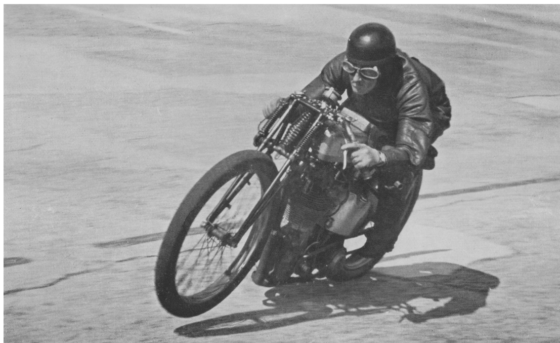
Figure 1. Noel Pope riding a Norton in a 500 cc record attempt, Brooklands, 1939. Note that the elevated front wheel does not have a front brake or front mudguard. Computer-enhanced scan from Full Chat, Plate 5 by Simon Kennedy.
