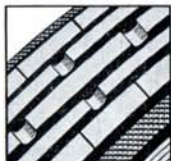
Interruptions in the centre ribs of the 'SPEEDMASTER' front tyre give good drainage and maximum braking.
